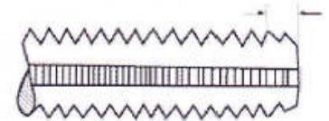
Bottoming Chamfer 1 - 2 Threads
