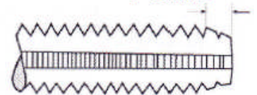
Modified Bottoming Chamfer 2 - 2½ Threads
