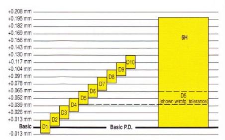
Again – the class of fit will give you maximum and minimum pitch diameter limits that need to be maintained during manufacturing. Within the class of fit – metric thread limits equal 0.013mm (0.013mm=0.00051"- extremely similar to that of fraction H limit tolerance.
