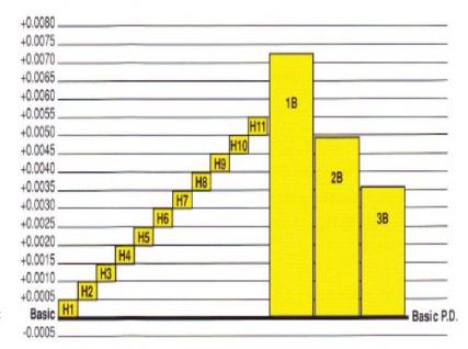
limits illustrated you are better able to understand what area of the class of fit you are actually working within. (This chart does not show a specific size tap – its purpose is to give visual understanding of how the "H" limits work within the different classes of fit)
